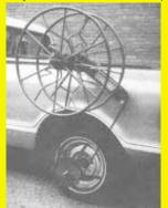
leys and a reel that mounts at one end of a steel shaft that mounts across the width of the pickup bed. The bottom pulley is fastened to a frame that attaches to the pickup wheel rim. The pulley sets out 10 in. from the center of the wheel hub and has adjustable spokes to fit different wheel sizes. A spring-loaded idler arm keeps the belt tight even when you go over bumps.
