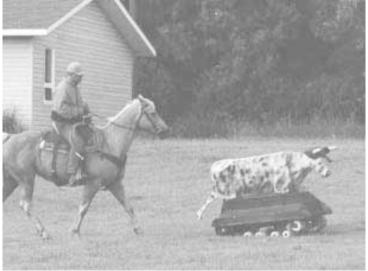
Remote control fiberglass steer mounts on Cat-type tracks and is fitted with two Honda 6 1/2 hp engines that each power a track.
