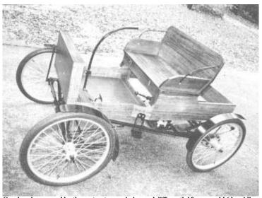
Carriage is powered by the motor, transmission and differential from an old 6 hp riding mower. It seats two people and has a stick tiller for steering.
