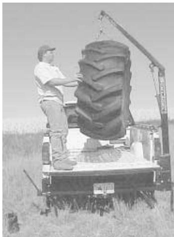
Self-contained hydraulic system uses two hydraulic cylinders. One raises the main mast up to a vertical position; the second raises the lift arm.
