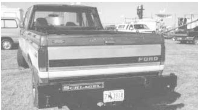
Heavy-duty bumper replaces pickup's original bumper. Hydraulic controls for hoist mount inside one end of bumper.
