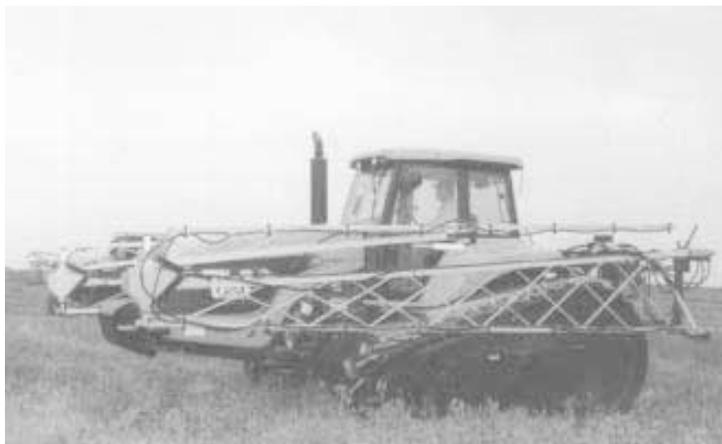
New 3-pt. mounted boom is designed for Deere and Cat Challenger tractors equipped with tracks set 120 in. apart. It folds forward to a transport width of 15 ft.
