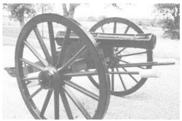
Rohlfing recently made this cannon which is mounted on 47-in. high wood wheels. It's based on an 1839 model used in both the Spanish American and Civil wars.
