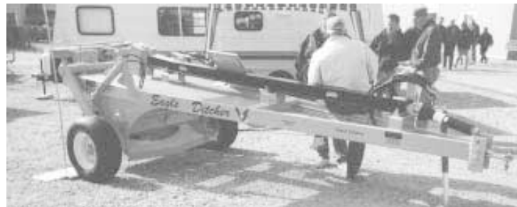
New ditcher uses a 4-ft. wide cutting blade to lift dirt and drop it onto a pto-driven flywheel that flings it outward. The design requires far less power to operate, according to the manufacturer.
