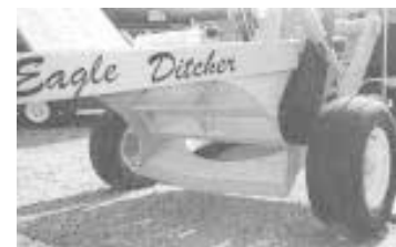
New ditcher uses a 4-ft. wide cutting blade to lift dirt and drop it onto a pto-driven flywheel that flings it outward. The design requires far less power to operate, according to the manufacturer.
