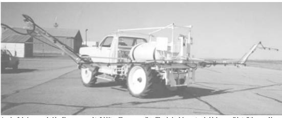
A pair of chains on each side of boom are used to fold it up like an accordion. The chain-drive system holds boom solid at all times and keeps it from bouncing up and down.
