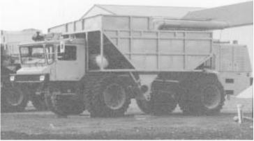
To build his 950-bu. grain cart, Lemieux started with a 4-WD airport fire truck. He stripped it down and built the big hopper from scratch.
