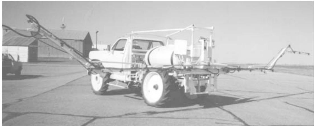
**A pair of chains on each side of boom are used to fold it up like an accordion. The chain-drive system holds boom solid at all times and keeps it from bouncing up and down.**
