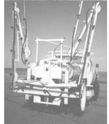
**Boom folds to a narrow 8-ft. transport width.**
