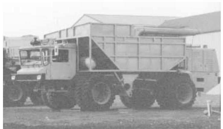
**To build his 950-bu. grain cart, Lemieux started with a 4-WD airport fire truck. He stripped it down and built the big hopper from scratch.**
