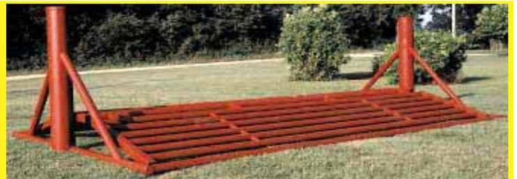
“No pit” cattle guard consists of two aprons mounted inside a steel framework. Coil springs are housed inside 6-in. dia. steel posts on each side of guard.
