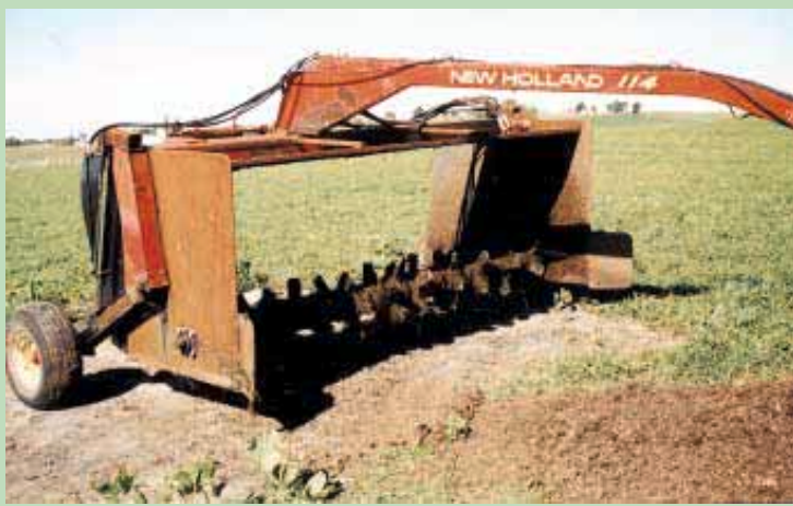
Callies's compost turner was built out of a New Holland Hydroswing Haybine frame.
