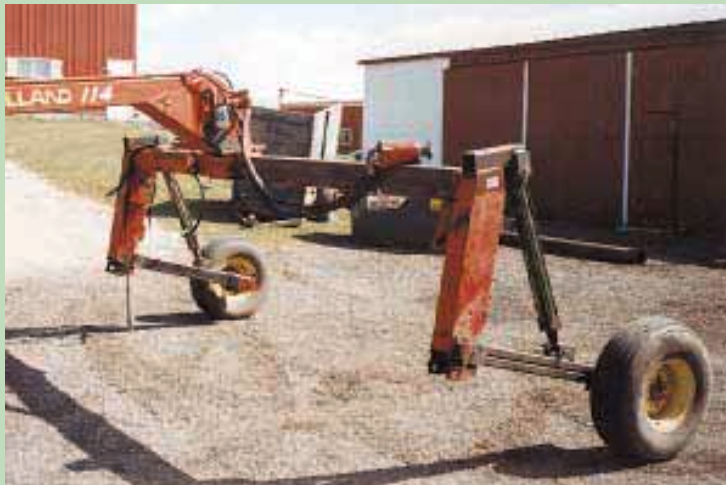
He widened the frame 3 ft., repositioned the wheels, and extended the arms that the wheels pivot on.
