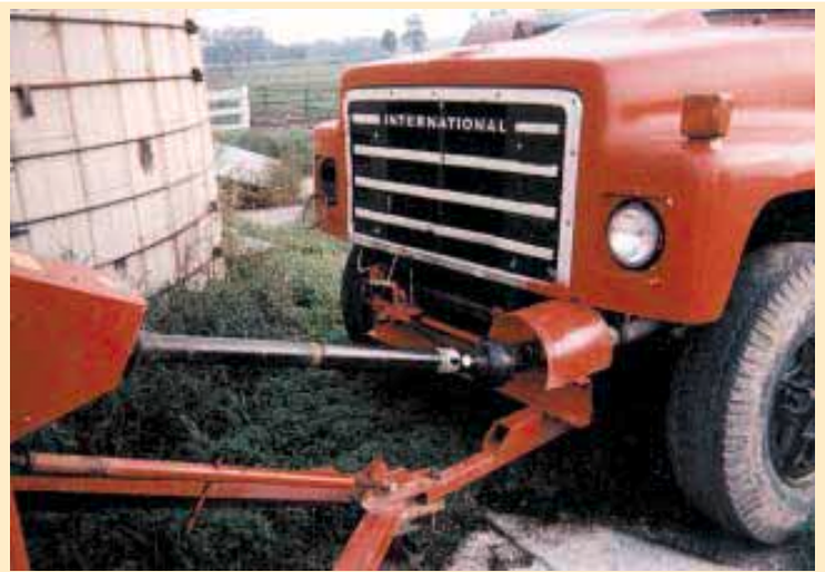
Dave Honderich converted the front end of an old IH truck into a portable power unit for pto work. He uses it to operate his silo blower and a manure pump.
