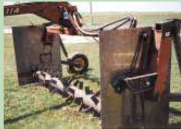
Rotor drum was fashioned from a heavy steel drainage pipe, with rigid flails welded to it at an angle.
