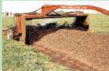
Unit will handle a pile of compost that's 4 1/2 ft. high by 12 ft. wide.
