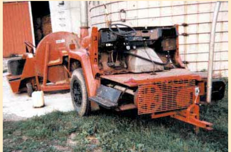
Cut-down truck has a hitch at each end and a jack under the back to support it when parked.
