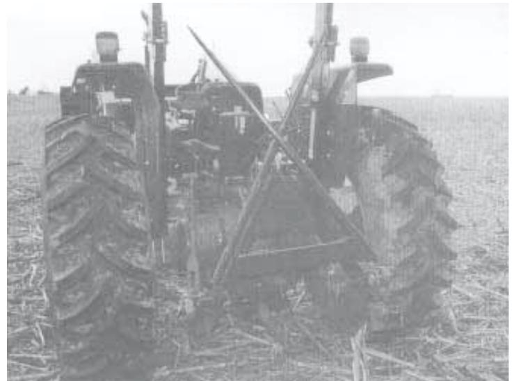
Double spears fold up out of the way, leaving drawbar accessible .
