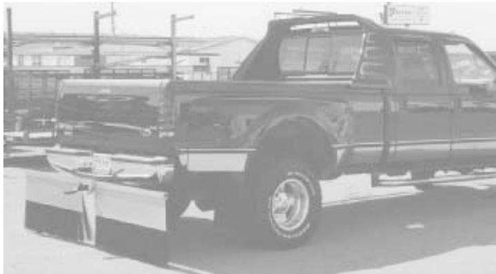
Full-width mud flap fits quickly onto a receiver hitch and locks in place with set screws in less than a minute.
