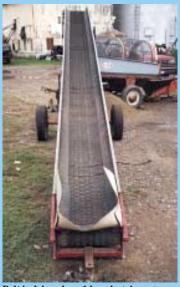
Belt is driven by a 1 hp. electric motor.
