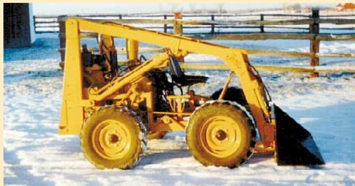
A matching pair of axles off Owatonna swathers was used to construct this skid steer loader. Lippert built everything, including the bucket and loader arms. Motor mounts at the back of machine for easy access.
