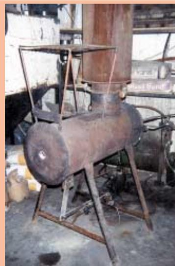
Water jacket wraps around flue, gathering heat which would otherwise go to waste. Heated water is pumped to trailer house. Note disc blade on end of stove which acts as a "safety valve".
