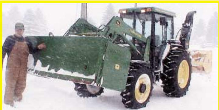
Campbell can push or pull snow, depending on how he sets the wings on the front-end blade.
