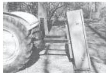
Bottom center part of box hinges on a pair of steel arms welded to a bracket that mounts on the 3-pt.
