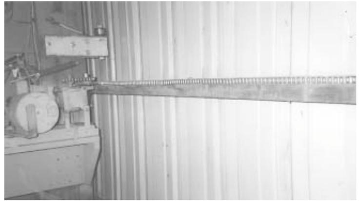
Automatic opener was made from a 1/3 hp motor salvaged from a garage door opener. It opens the 16-ft. door on Brandenburg's shop.
