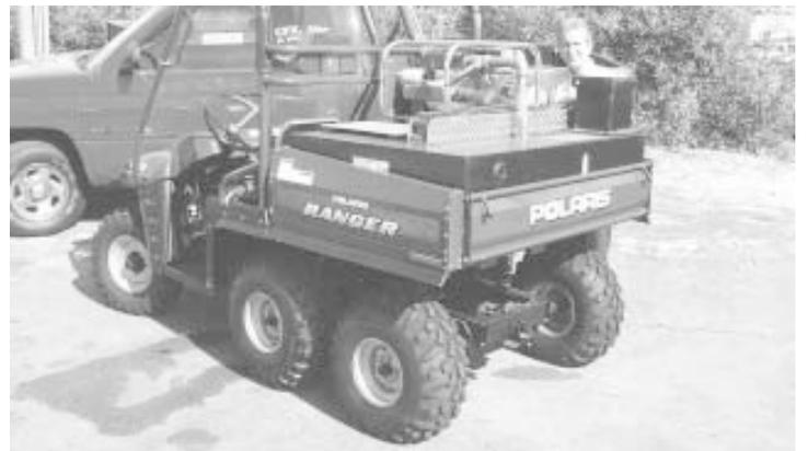
CFX Fast Attack ATEV (all terrain emergency vehicle) mounts on a Polaris ATV. Its pumping unit can move about 100 gal. of water per minute.
