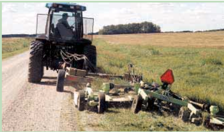
Extending a cylinder on the Handy-Hitch moves trailing mowers off the road and into the ditch.
