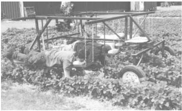
Self-powered cart holds four pickers laying on their stomachs.
