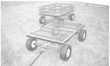
"Mini wagons" mount on flotation tires and carry loads up to 1,500 lbs. They're available with metal or wood racks.
