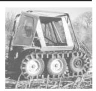
Rig's tracks are friction-driven by three sets of axles equipped with 15-in. tires.
