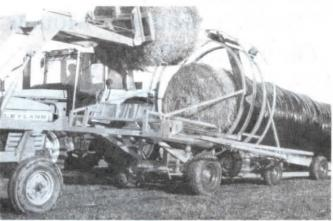
We at New Perth Agritech have acquired distribution rights to Grays Tube-Line bale wrapper from England which was first featured in FARM SHOW (Vol. 11, No. 5). The Tube-Line bale wrapper wraps an entire line of bales in one long continuous line. We've used one on our own farm for the past two years and find it to be a very fast wrapper designed for medium to large-sized opera-
