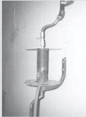
**Air hose runs through hole cut into side of pipe and up to quick coupler.**
