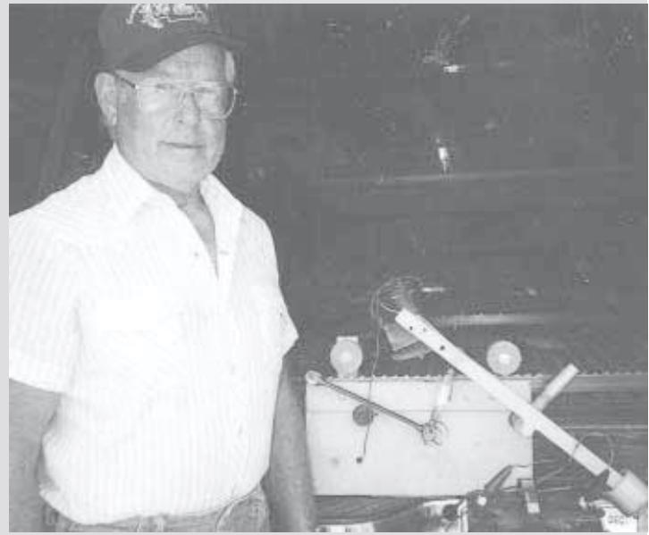
Witulski's blade sharpener uses a small grinder wheel that runs off a 12-volt motor.
