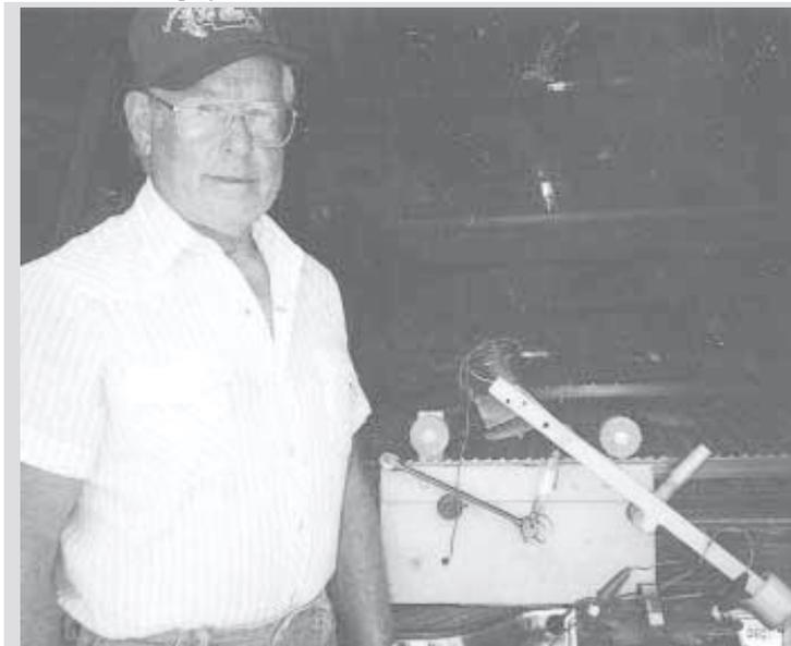
Wituski's blade sharpener uses a small grinder wheel that runs off a 12-volt motor.
