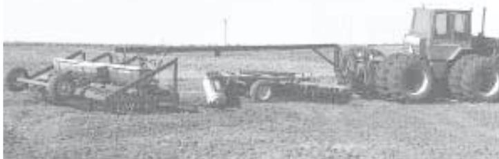
Gooseneck hitch is 27 ft. long and pulls Juhnke's home-built 18-ft. grain drill.
