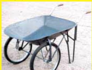
something I built recently, entirely out of junk parts. It's a wheelbarrow with bike wheels. I found the shell of a wheelbarrow without handles or wheels, and fitted it with the big wheels and a framework off an old exercise machine. It's much easier to roll around than a regular wheelbarrow. (**Roger Kuntz, 5251 County Road X, Grainfield, Kan. 67737**)
