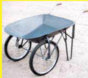
something I built recently, entirely out of junk parts. It's a wheelbarrow with bike wheels. I found the shell of a wheelbarrow without handles or wheels, and fitted it with the big wheels and a framework off an old exercise machine. It's much easier to roll around than a regular wheelbarrow. **(Roger Kuntz, 5251 County Road X, Grainfield, Kan. 67737)**
