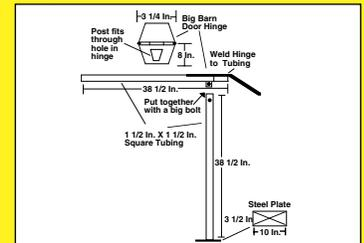
loose end hanging out over the end. I cut a hole in the hinge that fits down over the top of posts. As you "jack" up on the
