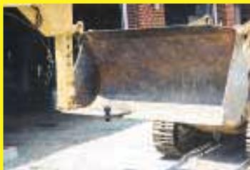
easier since I mounted a ball on my hi-lift bucket. I simply attached a metal drawbar to the front lip of the bucket and mounted a ball on that. It's easy to move trailers around. **(Charles W. Ballein, 1302 East national Pike, Scenery Hill, Penn. 15360 ph 724 945-5289)**
