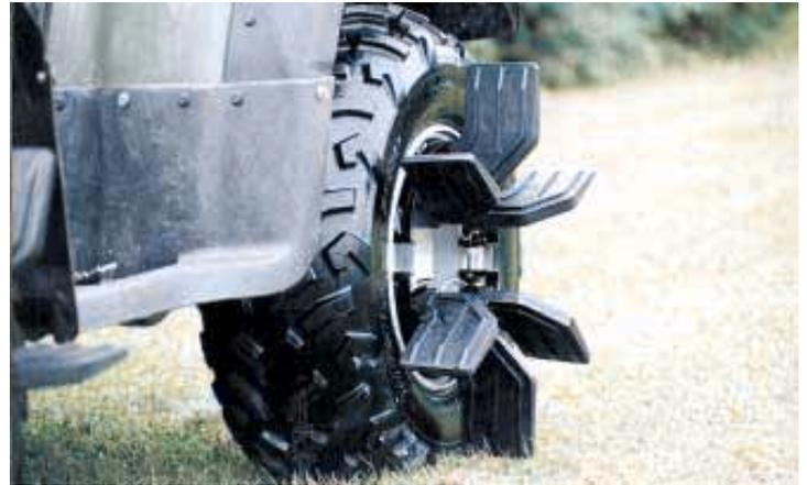
Mud paddles attach to a rim that fits tightly inside wheel rim. Paddles pull through mud and snow but are out of the way on dry ground.
