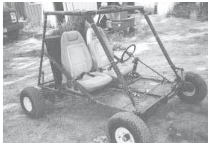
This heavy-built 6 1/2-ft. long, 74-in. wide go-cart is equipped with two bucket seats out of a Ford pickup, allowing it to comfortably seat two adults.
