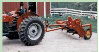
Teeth for the auger-shaped rake are spaced around a 4-in. pipe. They pick up and windrow rocks up to 10 to 12 in. in size.
