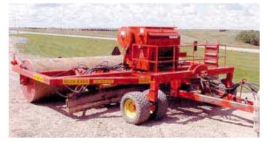
The 20-ft. wide "roller blader" is equipped with a pair of 10-ft. "swing blades" that can be angled forward or backward. Gauge wheels on front and back keep blades level.
