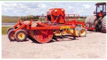
A Valmar air applicator mounts on top of machine, distributing seed between blades and roller on back. A 4-ft. dia. steel roller follows behind blades to press seeds into soil.
