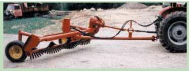
Geer built this rock rake using parts from an old New Holland Super 66 baler.
