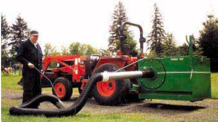
Pasture vacuum has a 22-in. impeller which provides enough suction to pick up manure, even in thick grass, and mulch it before blowing it into a hopper.
