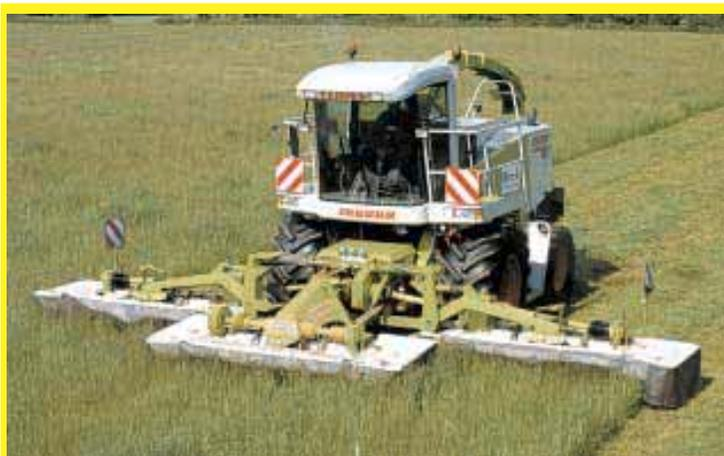
Claas 8500 C, a 3-section 30-ft. mower, mounts on front of the company's Jaguar self-propelled forage harvester.
