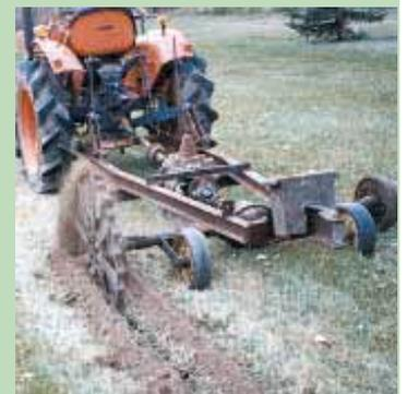
Rig makes a neat trench that's 8 in. deep and about 1 1/2 in. wide. A pair of rubber wheels on back regulate digging depth.
