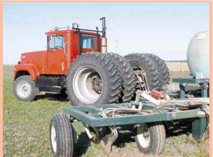
Fitting the tractor with dual wheels was one of the biggest challenges, say the Oetkens. They made wheel spacers out of 30-in. dia. natural gas pipe.
