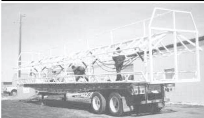
New “double decker” hay hauler is designed to fit any 45-ft. long semi trailer and consists of two cradles. Top cradle is hydraulically tilted down for loading.
