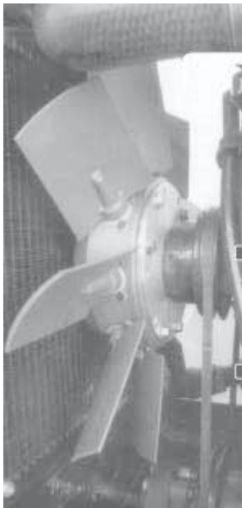
**A small 12-volt air compressor is used to change angle on fan's blades by 90 degrees, allowing fan to blow out instead of suck in.**
