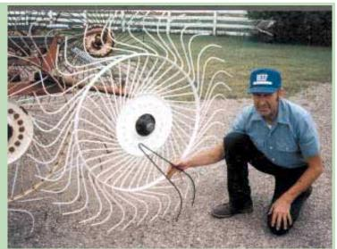
"It uses a trailing action rather than pushing into the direction of travel," says Mel Kuehn about his new "camber twin hay rake tooth?
