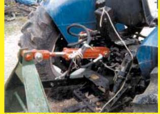
Seltzer cut a pair of steel brackets that pin to each end of cylinder. Brack-ets in turn pin onto tractor and 3-pt. hitch.
