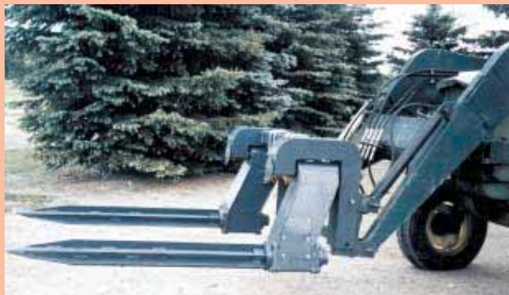
Hydraulic-driven tines have welded-on traction bars that grab bale as it’s being unrolled. Operator hydraulically moves tines closer together as bale gets smaller.
