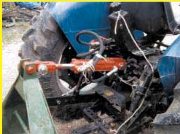
Seltzer cut a pair of steel brackets that pin to each end of cylinder. Brackets in turn pin onto tractor and 3-pt. hitch.
