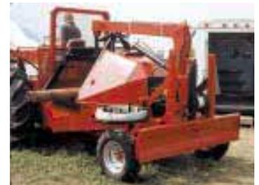
Hydraulic-controlled blade on back of machine is used to clear fence rows before beginning work, and also to pull fence posts.
