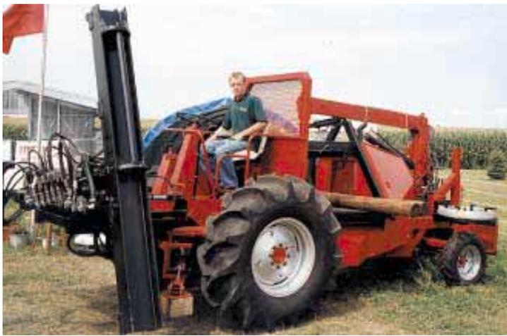
Up-front post driver tilts hydraulically in any direction and mounts on a telescoping table that extends 3 ft. out to the side and 3 ft. to the front.
