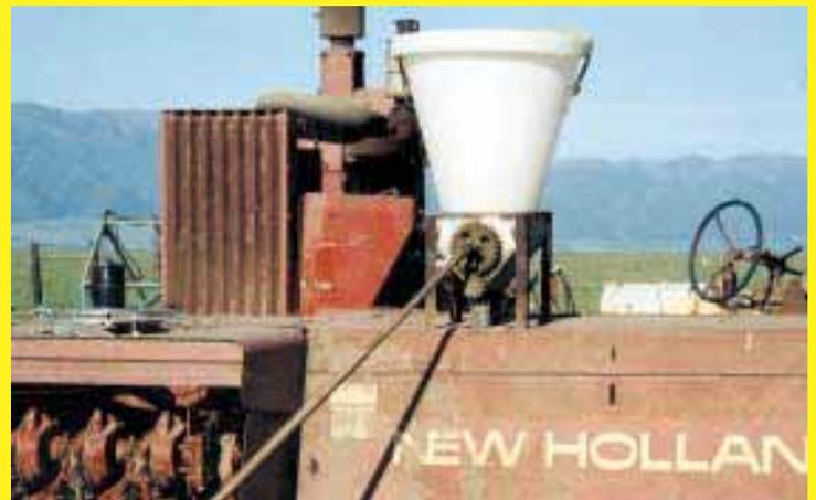
La Macchia injects clover and other grass seed into bale chamber as he bales. A pair of rubber tubes run from hopper through holes cut into baler.
