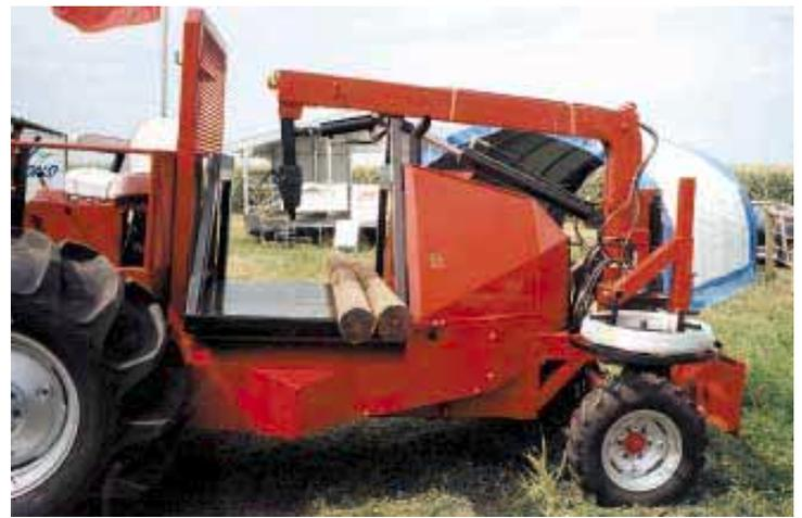
A lift arm loads posts onto carrying platform at center of machine. Platform tilts hydraulically to the side to make it easy to unload.
