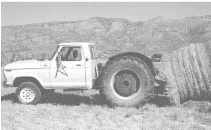
**“Trucktor”** consists of the back half of an IH WD-9 tractor and the front half of a 1978 Ford F-250 1-ton pickup. Inventor Frank Mayo often uses it to haul round bales.
