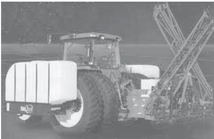
Demco's high capacity saddle tanks mount on extended rear axle spindles that shift weight to the rear, relieving stress on the tractor's front axle and chassis.
