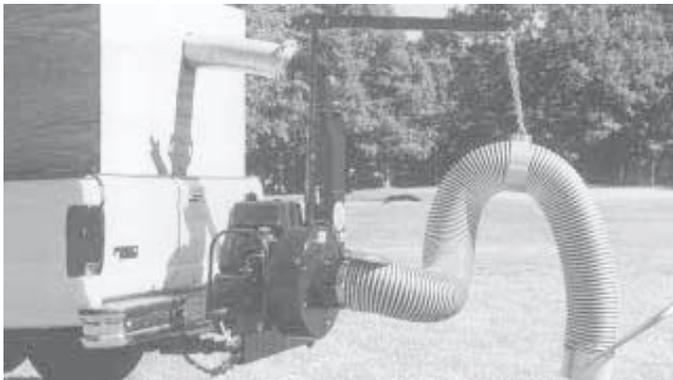
Leaf vacuum hooks up to receiver hitch. A 10-ft. long flexible hose sucks debris up into hopper on pickup bed. Suction fan is driven by its own auxiliary engine.
