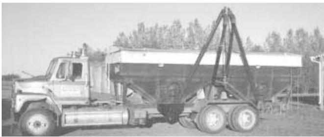
Tandem axle truck is equipped with two 325-bu. Unverferth gravity boxes, as well as two drill fill augers.
