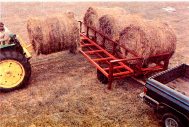
Bale spear loads bales onto "non-hydraulic" bale cradles that unload bales without the need for tractor hydraulics.
