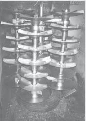
glance. I removed the gangs and welded short lengths of angle iron to the bearing holders on all the gangs. I welded two gangs to a pipe opposite each other. The next two gangs are welded opposite each other but are lower than the two gangs welded to the pipe. The stand that holds the rack upright is the rear wheel of a disker which has weights on it.
