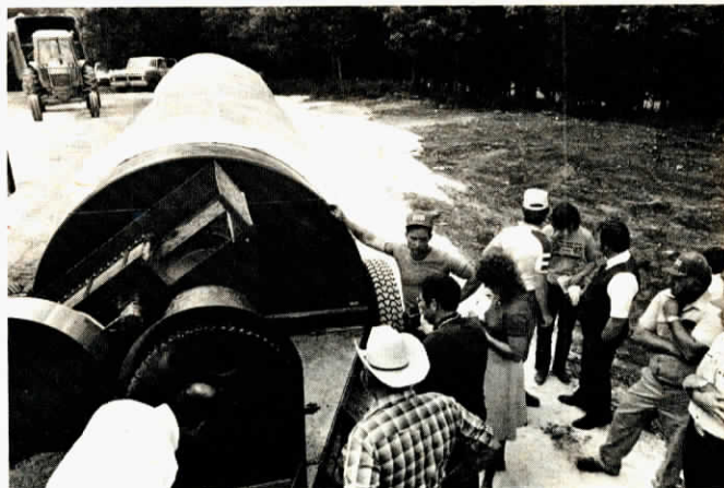
The Porta Packer fills bags with a 20-in. dia. earth auger that'll handle "almost any free-flowing material".
