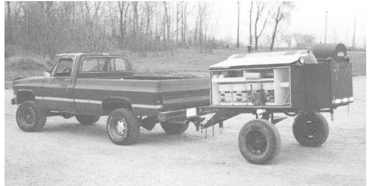
Converted sprayer still has the original spray tank. Harris mounted a 6-ft. long wooden storage compartment on one side of it and a smaller compartment behind it.
