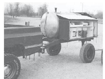
Both compartments have hinged lids that can be lifted up out of the way.
