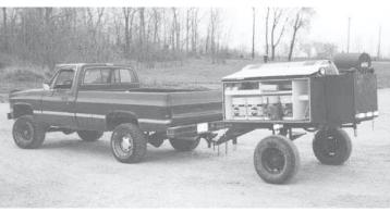
Converted sprayer still has the original spray tank. Harris mounted a 6-ft. long wooden storage compartment on one side of it and a smaller compartment behind it.
