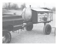
Both compartments have hinged lids that can be lifted up out of the way.
