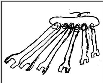
pile because the holders that come with them don't work well. I just thread them onto a 12-in. piece of #12 copper wire. The wire is soft enough to bend easily, yet strong enough to hold its shape and hook together.
