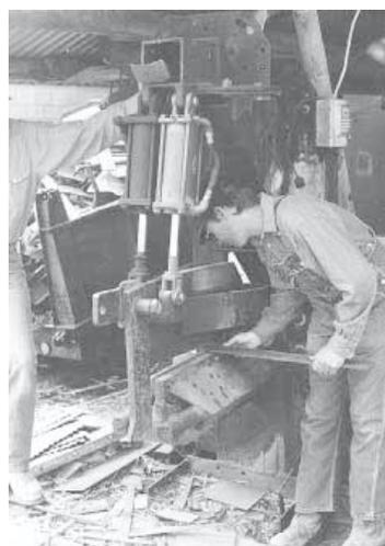
Top part of Ray's shear is raised or lowered by a pair of large diameter hydraulic cylinders.
