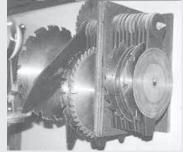
way to keep them in good order. He came up with a wall-mounted storage bracket with twenty swinging arms that each hold a blade. The arms hang freely from a long bolt that runs through a plywood brace at the center of the bracket. The blade hangs loosely on a peg at the middle of each arm. The arms extend down below the blade so you can grab it with your hand, swing it up, and pull the blade off. The entire blade holder takes up only about 2 sq. ft. of wall space.
