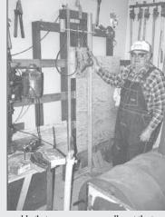
a cable that runs up over a pulley at the top. A weight on the cable is slightly heavier than the saw so it moves easily up and down. A bit of down pressure is all that's needed.
