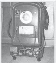
of Bridge diodes mounted on a panel that can be mounted inside a steel frame and fitted with caster wheels so the welder can mount on top of it. Sells for \$225. The panel alone (without the frame and caster wheels) sells for \$125 to mount on the side or top of the welder.
