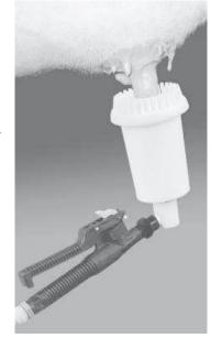
Teat Foamer solution is pumped from a canister set up in milk house through lines to drops fitted with application cups. Foaming pre-dip covers teat completely and clings to udder without dripping until wiped off with a towel. (Sani-Sure also sells inexpensive cloth dairy towels that they say clean and dry udder better than paper. They also cost 60 to 70 percent less to use, according to the company.)
