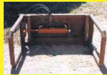
make the rest of the frame. One of the arms is opened or closed by a 16-in. long hydraulic cylinder that extends horizontally across the front part of the frame. The other arm is held rigid by a length of chain that's welded to the side of the frame. If necessary, the angle of the rigid arm can be changed by repositioning the chain in a notched hole in the frame.
