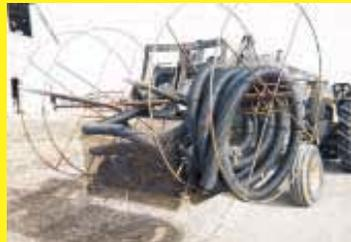
that mounts over the bale loader on my front-end loader. We made a metal framework for each reel to connect it to the pipe. With two reels we can carry two different sizes of tile. For example, we can haul 150 ft. of 6-in. tile on one reel and 250 ft. of 4-in. tile on the other reel. The reels are supported by steel I-beams originally used by phone or electric companies to support large reels of cable. Each reel slips onto the pipe and is held on with a piece of chain.
